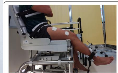
Fig. 3 Experimental setup for the measurement of isometric strength and voluntary activation of the quadriceps femoris muscle
